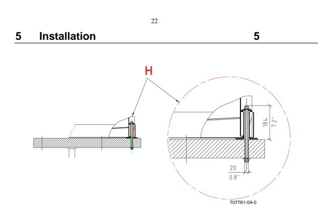
H \_\_\_\_\_Ceiling bore holes (20 mm or 3/4 in ∅) for through bolt, length depending on the thickness of the ceiling. Support if necessary
