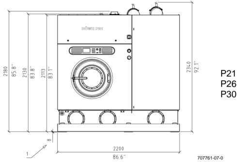
1= With the legally stipulated floor clearance of the safety trough, the machine height increases by the size of the spacer plate (8 mm/.3 in).
