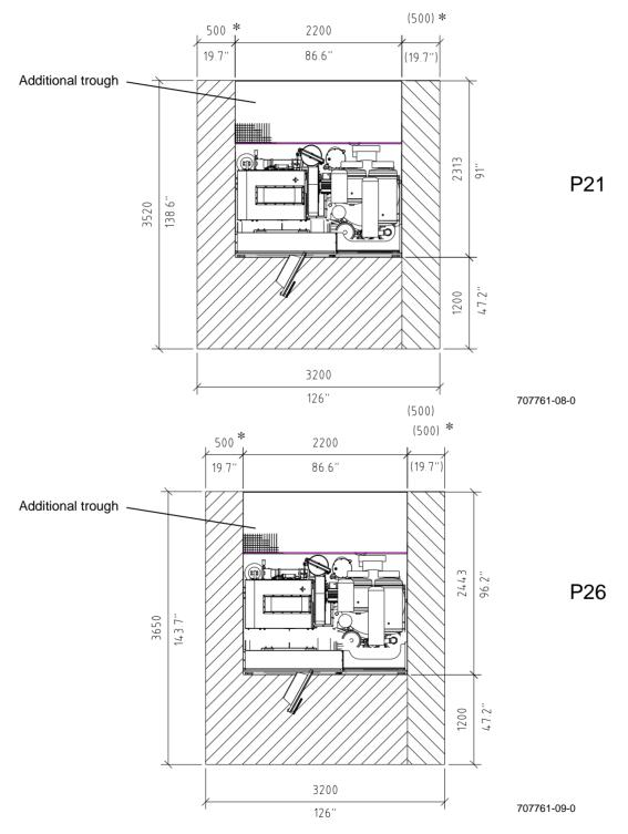
\* The machine can be placed at the wall either at the left or right hand side.
