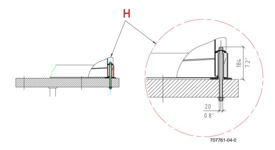
**H** \_\_\_\_Ceiling bore holes (∅ 20 mm or 3/4 in) for through bolt, length depending on the thickness of the ceiling. Support if necessary
