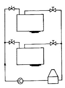
When supply and drain lines are fitted with hand valves, both valves must be opened before starting the machine, so that cooling is ensured and the sensor in the condensate drain line of the still responds in case of cooling water shortage.
