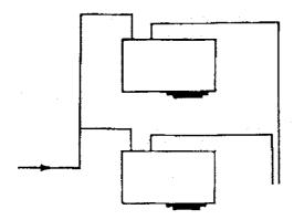
Cooling water drains must be separate.
