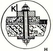
Ceiling borehole 20 mm °) for through-bolts, length depending on thickness of ceiling. Support if necessary.
