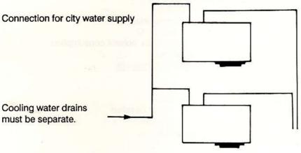
Connection with water recirculation (refrigeration unit or cooling tower)
