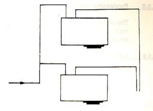
Cooling water drains must be separate.
