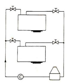
When supply and drain lines are fitted with hand valves, both valves must be opened before starting the machine, so that cooling is ensured and the sensor in the condensate drain line of the still responds in case of cooling water shortage.
