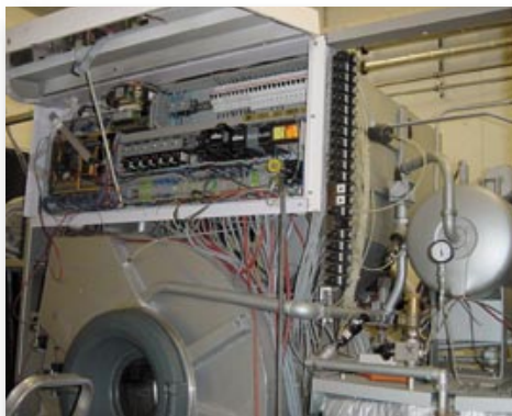
Testing procedure of a dry cleaning device on one of our test-benches
