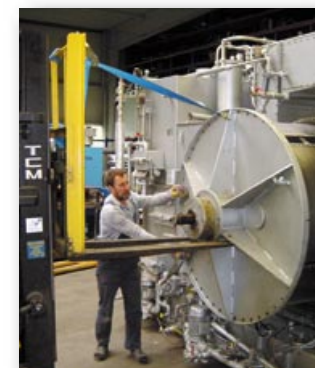
Replacing the main bearings in a BÖWE industrial dry cleaning machine
